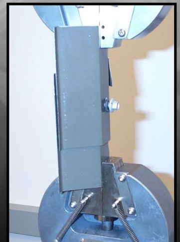
Lab equipment utilizes high-frequency vibrations to simulate thermal expansion and contraction.
